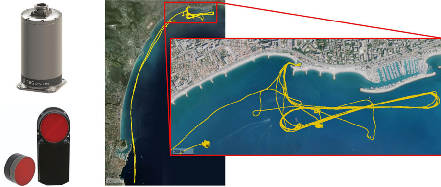
FIGURE 14 Top left: Apogee IMU subsea; bottom left: Teledyne Pathfinder DVL; right: 6-h-long acquisition in southern France with an Apogee IMU and a Teledyne DVL
