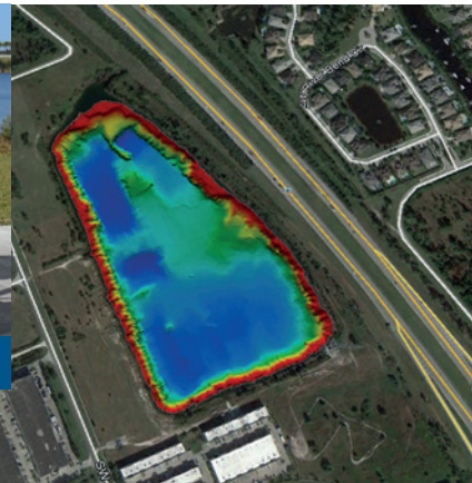
Bathymetry data collected with the USV 2.5
